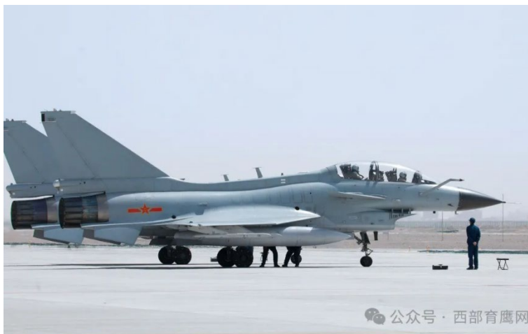
A J-10S at the Xi'an Flight Academy. The J-10S is a two-seat version of the J-10 fighter.
